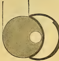
FIG. 15. WARWICK RIM, COMPRESSED CUSHIONED TIRE. Dotted lines show amount of rubber exposed for use.
